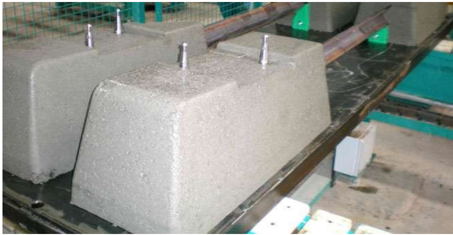
Dual Block Concrete sleepers
