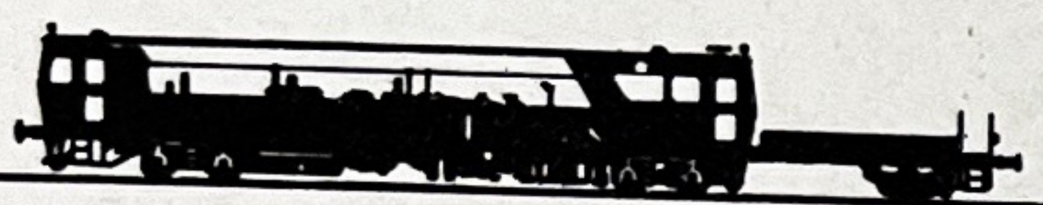
08-32 Levelling, lining and tamping machine
