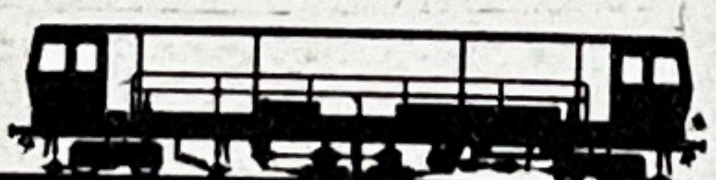
DGS 62 N Continuous action Dynamic Track Stabilizer
